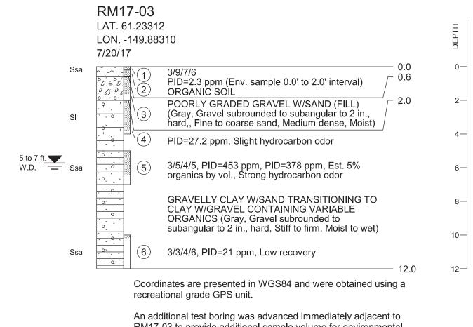
RM17-03 to provide additional sample volume for environmental sample collection. The two holes are treated as a single exploration.
