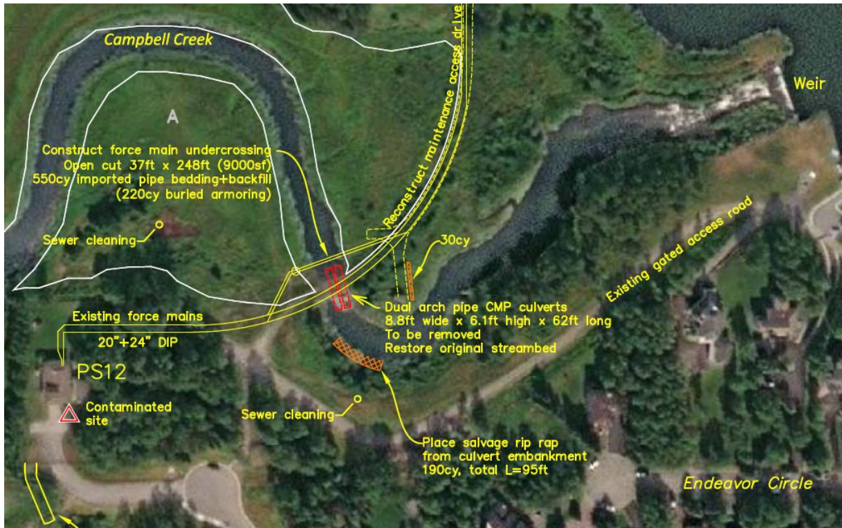
Figure 1: Project map submitted by the applicant showing the work to be completed (highlighted in yellow). The spur road and turn-around are drawn emanating from the existing maintenance path, and the culverts proposed for removal are highlighted in red.
