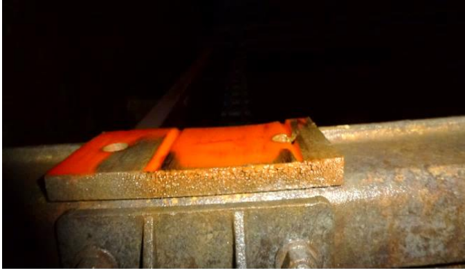
Figure 4-9 North Sediment Basin – Worn Basin Wear
