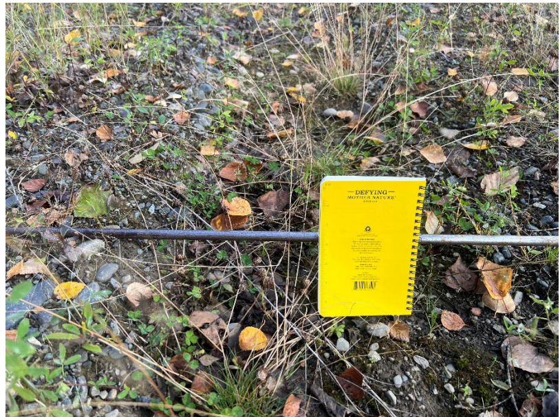
Close up image of typical ground cover and approximately 3.5-inch rut using probe rod for reference.
